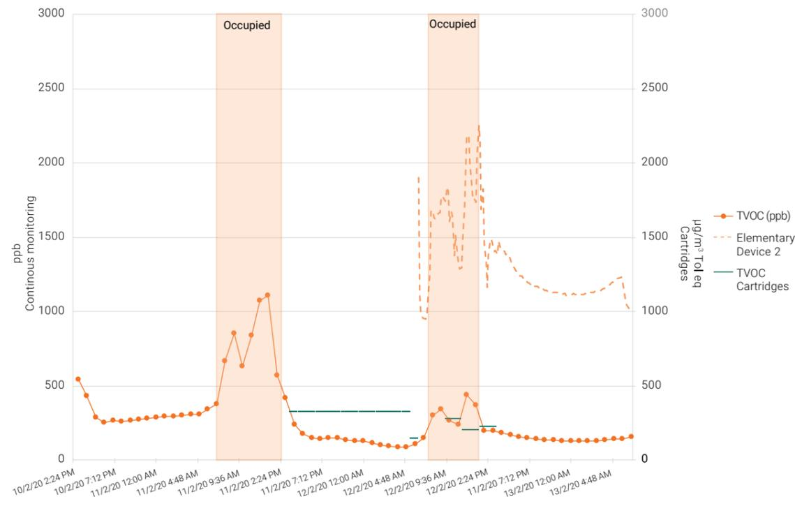
**Figure 10: Comparison between continuous monitoring and samplings on cartridges over the study in the kindergarten class.**
