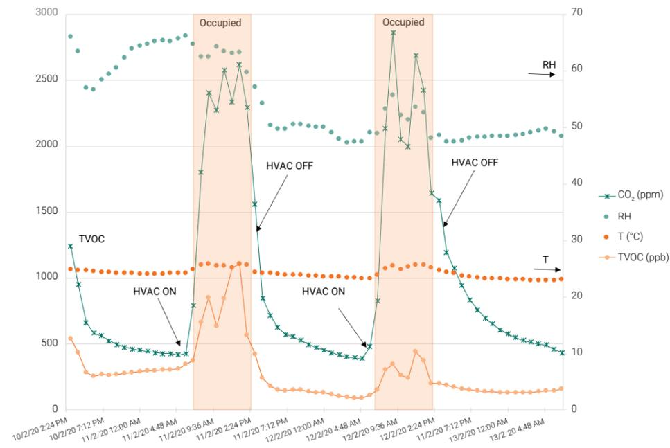
**Figure 7: TVOC variations (in ppb) comparison in between the three monitored room: empty room (ground floor), kindergarten room (ground floor), elementary room (first floor); "Occupied" area represent the class hours; HVAC system switch ON/OFF are indicated by a black arrow;**
