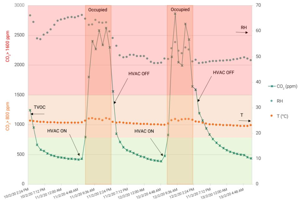
**Figure 4: T°, RH and CO<sub>2</sub> continuous monitoring in the kindergarten classroom; Occupied period dark green area on the graph, Black arrow indicates HVAC system switch ON/OFF; three colors highlight different levels of comfort zone for CO<sub>2</sub>: green-Comfortable; Orange-Uncomfortable; Red: Critical**
