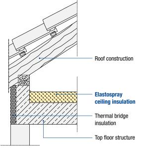
Insulation to the floor of an unheated loft/attic space
