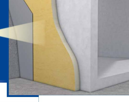
The external walls of buildings usually make up the largest surface area through which heat can escape. Between 100 and 150 kilowatt hours of heating energy escape annually through one square metre of un-insulated wall. This equals approximately 10 to 15 litres of fuel oil or 10 to 15 cubic metres of gas. Basement walls, despite not being visible, are external walls. External thermal insulation (perimeter insulation) of basement walls with Elastospray can reduce energy consumption by up to 90 %.
