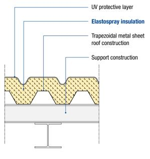
Trapezoidal metal sheet roof with external insulation and UV protective layer
