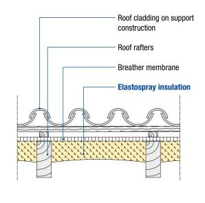
Rafter roof with membrane and internal between-rafter insulation
