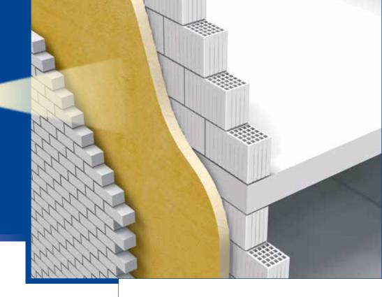
Many buildings are designed with double skin masonry for visual or structural reasons or as protection against extreme weather conditions. The cavity is given an insulating layer so that the cold air between the facing wall and the lining wall does not then cool the external wall and therefore have a negative effect on the energy consumption of the building.
