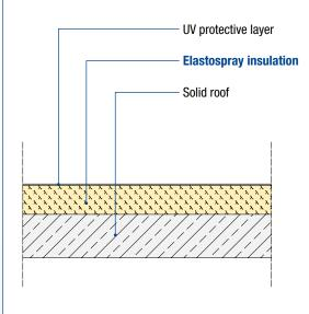
flat roof with external thermal insulation and UV protective layer
