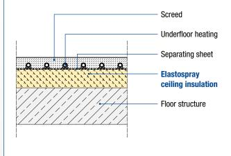
Insulation under the heating screed
