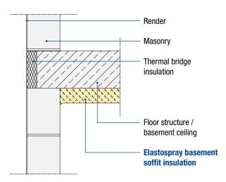
Soffit insulation for unheated basements
