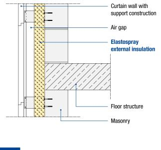
External wall with thermal insulation and curtain ventilated cladding
