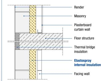
External wall with internal insulation and a lightweight or solid facing wall
