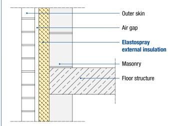
Double skin masonry with core insulation and air gap
