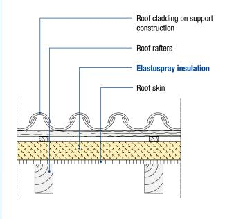
Rafter roof with visible rafters,top roof skin and external thermal insulation
