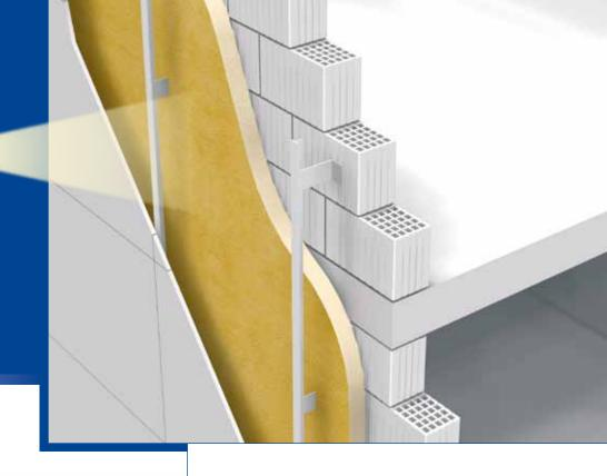
The external insulation behind a curtain wall or with ventilated cladding can be used both in new buildings and refurbishment of existing buildings. The cladding protects the external components against weathering and as a decorative facade gives a designer, lots of options
