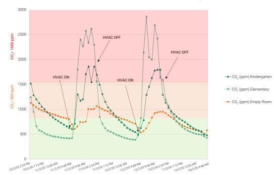
Figure 5: CO<sub>2</sub> concentration comparison in between the three monitored classrooms: empty room (ground floor), kindergarten room (ground floor), elementary room (first floor)
