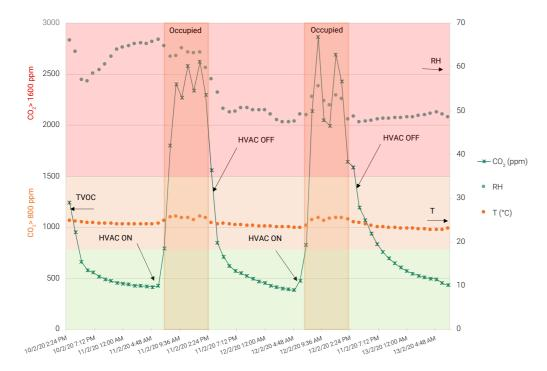
Figure 4: T°, RH and CO, continuous monitoring in the kindergarten classroom; Occupied period dark green area on the graph, Black arrow indicates HVAC system switch ON/OFF; three colors highlight different levels of comfort zone for CO,: green-Comfortable; Orange-Uncomfortable; Red: Critical
