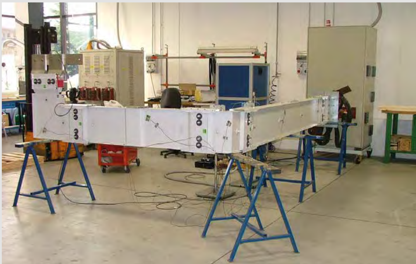
The Zucchini lab during the tests for the approval certification of SCP busbar trunking systems
