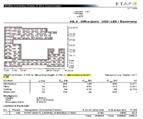
Specific connected load: 2.60 W/m² = 0.97 W/m²/100 lx (Ground area: 953.48 m²)
