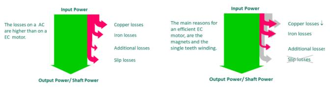
Figure 2 Power losses of an AC Motor (left) compared to the power losses of an EC Motor (right).
