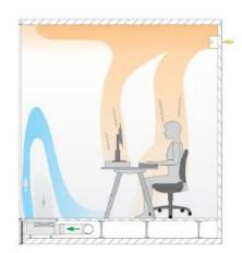
Figure 4 : Floor Induction Cooling
