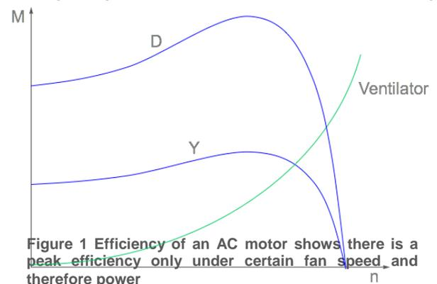
efficiency, which drops considerably at either side of the optimum operating point as shown in Figure 1.
