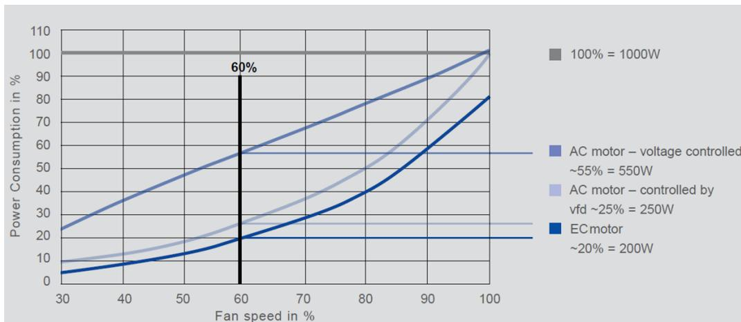
Figure 3 shows that an EC motor consumes less power than AC motors whilst operating even at 20% fan speed.
