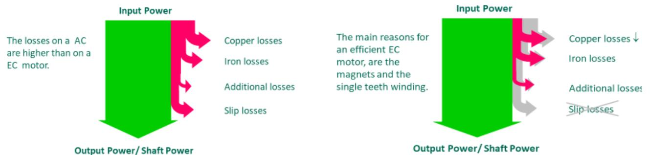
Figure 2 Power losses of an AC Motor (left) compared to the power losses of an EC Motor (right).
